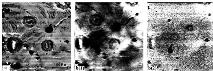
**Fig. 1.** Images of phoenix leaf: (a) SEM image; (b) SEAM images at  $f = 184$  kHz: (1) amplitude image; (2) phase image.
